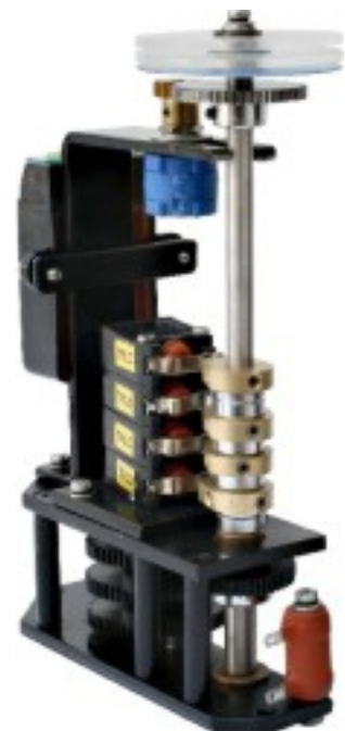
Travel Switch arrangement
