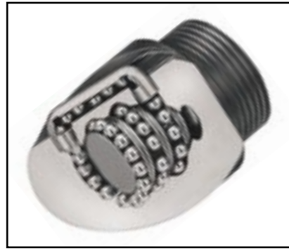
Rolled thread ball screw with ball recirculation by integrated tube.
